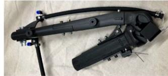
3D printed leg assembly with femur, knee, tibia, patella. Extensor BPA is connected while the flexor BPA is disconnected.
