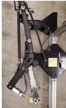
3D printed leg assembly fixed in the test stand for isometric torque test. Flexor BPA is attached and inflated, while the extensor BPA is detached. Load cell is mounted at a right angle to the tibia and attached to a swing arm.
