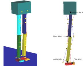
(a) Bipedal walker model showing the size body segments: pelvis, thighs, shanks, feet, and toes. (b) Bipedal walker model with joints labeled. Antagonistic muscle pair are color-coded: red for flexors and blue for extensors.
